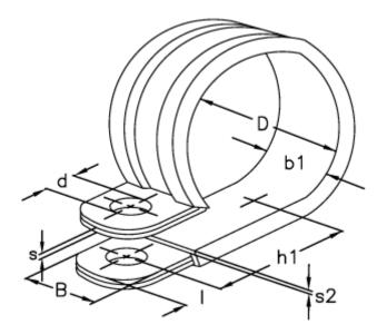
$\begin{array}{lll} b1 & = 18.5 \\ d & = 6.4 \\ Diameter D = 22 \\ h1 & = 22.2 \\ I & = 6.0 \\ s & = 0.80 \\ s2 & = 1.5 \\ Width B & = 15 \\ \end{array}$
